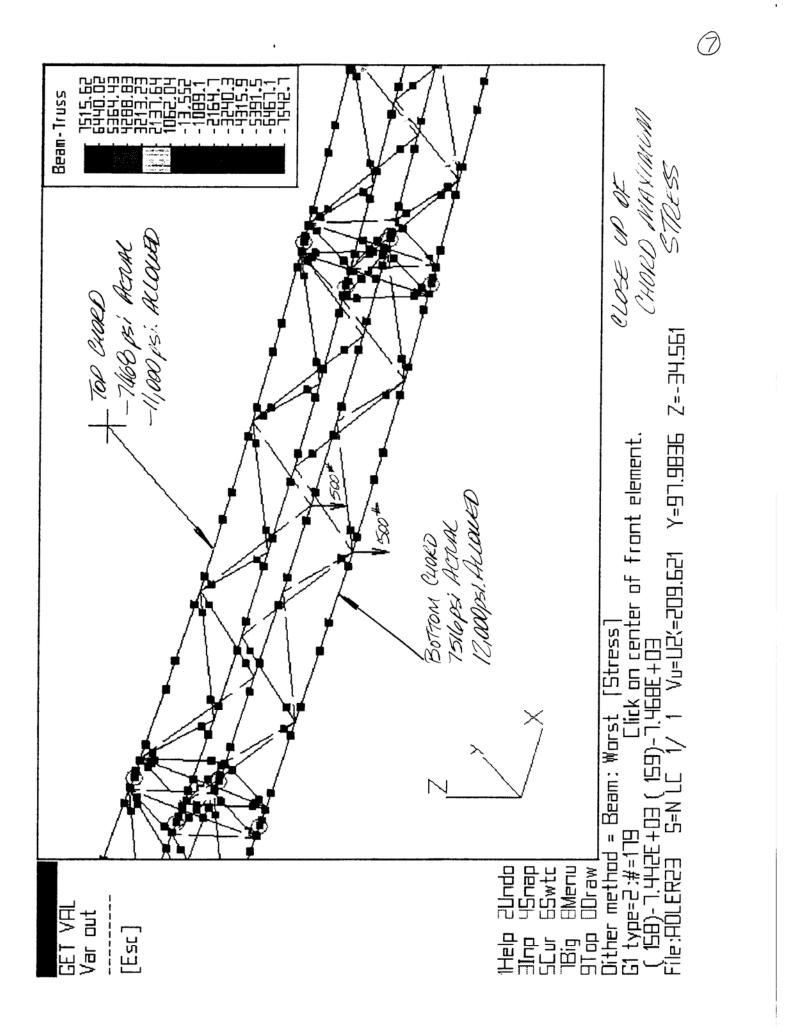
B 1576896 BUCKLING CALCULATION A= • 7363 in Z" O.D. ×<sup>1/</sup>BUAU  $T = 0.650 \text{ in}^4$ I = -325 m2= ·325 in 4  $K = \int \frac{d^2 + d_1^2}{16}$  $k = \sqrt{\frac{2^2 + 0.75}{4}^2} = -164$ EULAR METHOD Var = ATTZET WHERE N=12 FOR FIXED-FIXED Per = 1.2(TT2)(10:3×10)(.325) Pcg = 44,051 # Pcp >> 4766 # ACTUAL. SINCE TRY SECANT FORMULA UTH VARIOUS ECCONTRICITIES
